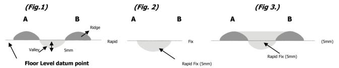
The illustration (Fig. 1) above shows a maximum and a minimum of 5mm in the levels. Thus between A and B a minimum of 10mm of product has to be poured to get the floor to the level of the highs at A and B.
