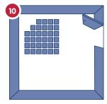
Tile out from the centre mark to the edges, keeping lines straight and tile spacing even. Leave cut tiles until last.
