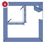
Mark the new starting point and transfer these marks to the corresponding skirting boards or walls. Position straight edges on these marks in both directions.
