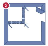
Starting at the centre mark, place a row of loose tiles along these lines. Cut tiles should be at least half a tile wide. If this is the case, position straight edges as per step 4. Remember to leave room for tile spacers, tile panel movement joints and perimeter joints.
