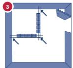
If cut tiles are too small, move the centre tile so that the middle of the tile coincides with the centre mark on the floor.
