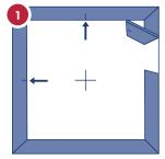
Determine the centre point of the room and mark it. Transfer these marks to the corresponding skirting boards or walls.
