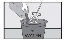
Mix 20kg TAL GOLDSTAR XL Tile Adhesive with 5I of cool water. Using a mechanical mixer, mix to a creamy lump-free paste, while adding powder.
