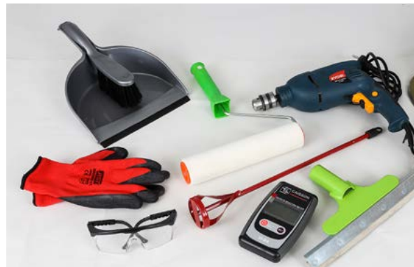
Broom, slow speed drill (350rpm), mixing paddle, short pile Mohair roller, moisture meter, rubber squeegee, PPE.
