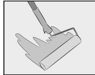
Apply TAL VAPORSTOP HB if prevailing moisture levels do not attain 5% (75% RH) or less.
