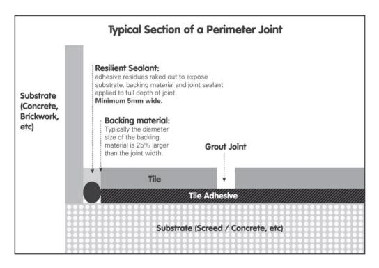
TAL Website : General Specification for Installing Under-Tile Heating Elements, and fixing Glazed Ceramic Floor Tiles or Porcelain Tiles
